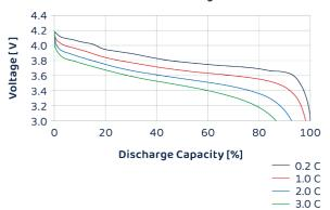
Charge: CC/CV: 2.0 C - 4.2 V (0.05 cut-off) at 25°C Discharge: CC: Different C-Rate to 3.0 V cut-off at 25°C
